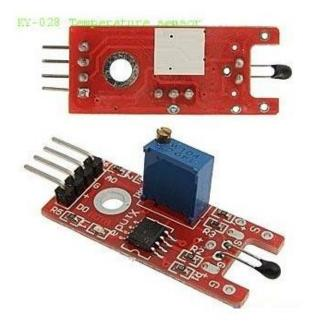
Simple circuit of digital temperature module and integrated LED connecting to digital 13 interface to make temperature indicator light.
